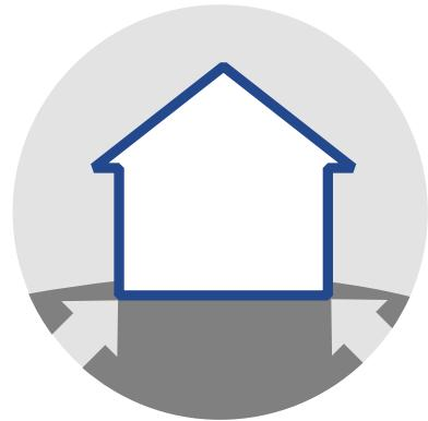
In climates with mild winters, slab insulation in a typical 1,800 square-foot home would save \$50 to \$60 annually. R-10 slab insulation for an 1,800 square-foot home would typically cost \$300 to \$600 to install. Thus, the insulation would pay for itself in 5 to 10 years.
