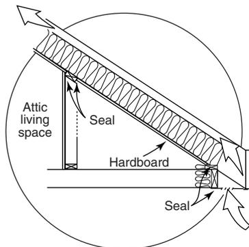
In new construction, an improved approach is to insulate and air seal the rafter space along the sloped ceiling of the knee wall. The rafters should be covered with a sealed air barrier, such as drywall, rigid insulation, or foil-faced hardboard. The advantage of this approach is that the storage area as well as all the ductwork is now inside a more tempered space.
