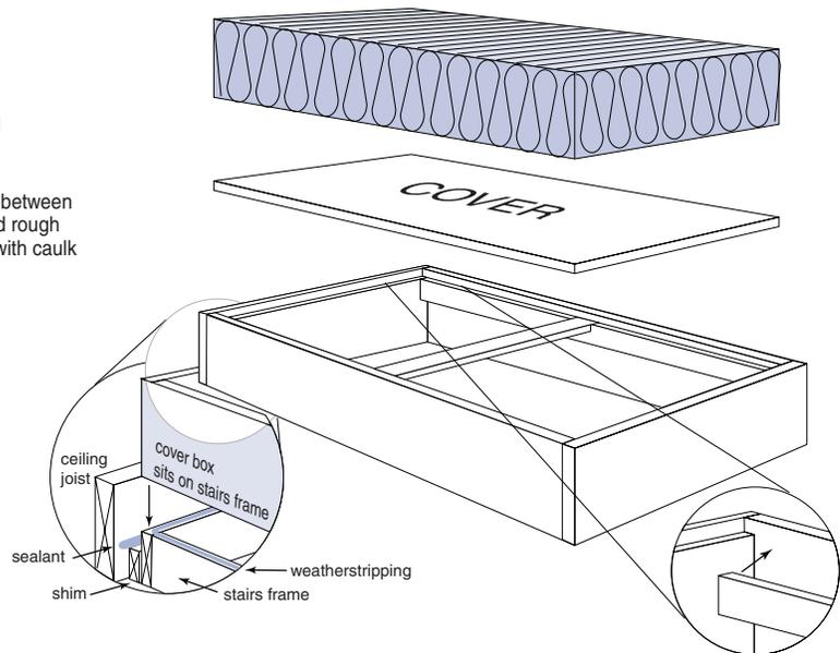
As with all home projects, follow manufacturer's instructions for proper installation of the attic stairs. These instructions often provide unique techniques and safety considerations for each particular unit. For safety and extended life of the stairs, be sure to cut them to the proper length. This action will avoid straining the hinges and reduce wear on the pivotal joints of the stairs.
